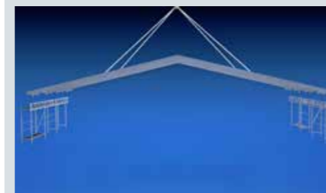
Positioning by crane onto a support base out of lattice girders
